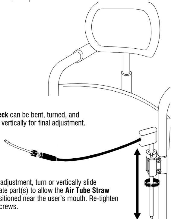
4. For final adjustment, turn or vertically slide appropriate part(s) to allow the **Air Tube Straw** to be positioned near the user's mouth. Re-tighten all cap screws.
