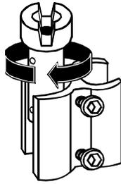
2. Place **Figure-8 Collar** with Sip-N-Puff unit onto chair frame, and tighten button head cap screws. The **Figure-8 Clamp** can be turned and adjusted vertically during final adjustment.
