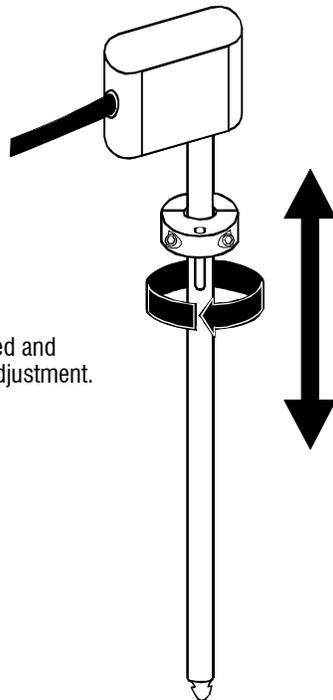
4. The pin in the **Pinned Split Collar** must rest in the notch in the **Notched Step Collar**.
