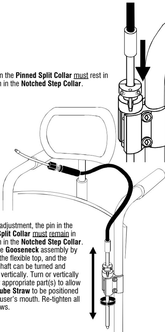
5. For final adjustment, the pin in the **Pinned Split Collar** must remain in the notch in the **Notched Step Collar**. Adjust the **Gooseneck** assembly by bending the flexible top, and the bottom shaft can be turned and adjusted vertically. Turn or vertically slide any appropriate part(s) to allow the **Air Tube Straw** to be positioned near the user's mouth. Re-tighten all cap screws.
