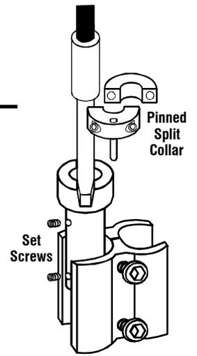
2. Place **Figure-8 Collar** with Sip-N-Puff unit onto chair frame, and tighten **Figure-8 Clamp's** button head cap screws. The **Figure-8 Clamp** can be turned and adjusted vertically during final adjustment.
