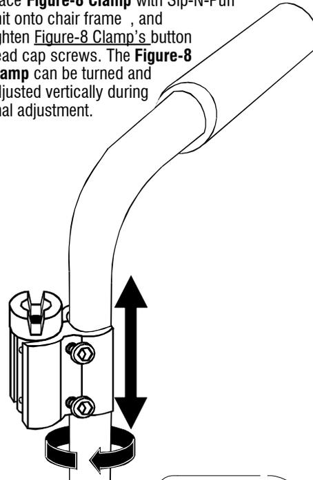
3. **Gooseneck** can be bent, turned, and adjusted vertically for final adjustment.
