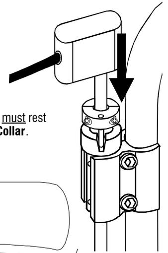
5. For final adjustment, the pin in the **Pinned Split Collar** must remain in the notch in the **Notched Step Collar**. Adjust the **Gooseneck** assembly by bending the flexible top, and the bottom shaft can be turned and adjusted vertically. Turn or vertically slide
