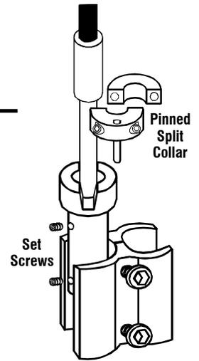
2. Place **Figure-8 Clamp** with Sip-N-Puff unit onto chair frame, and tighten **Figure-8 Clamp's** button head cap screws. The **Figure-8 Clamp** can be turned and adjusted vertically during final adjustment.
