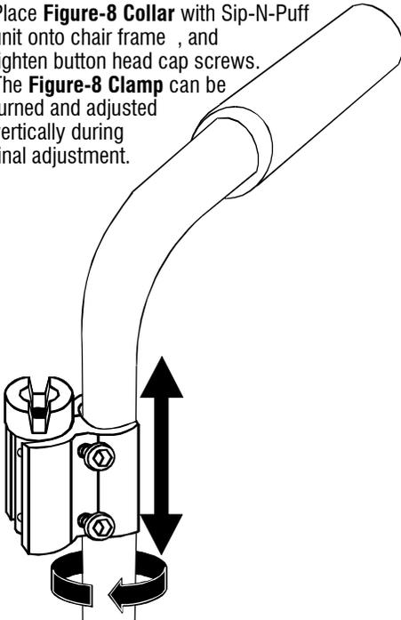
3. **Pinned Split Collar** can be turned and adjusted vertically during final adjustment.
