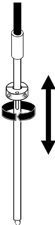
4. The pin in the **Pinned Split Collar** must rest in the notch in the **Notched Step Collar**.
