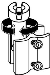
2. Place **Figure-8 Clamp** with Sip-N-Puff unit onto chair frame, and tighten button head cap screws. The **Figure-8 Clamp** can be turned and adjusted vertically during final adjustment.
