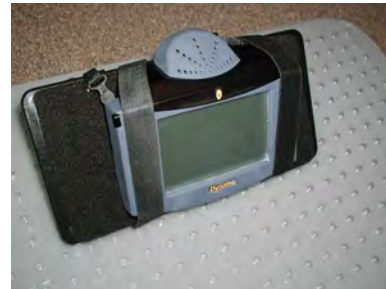
Small voice output device strapped securely onto angled block in front of student
