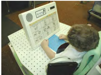
Large communication device securely positioned at 60 degrees in front of student
