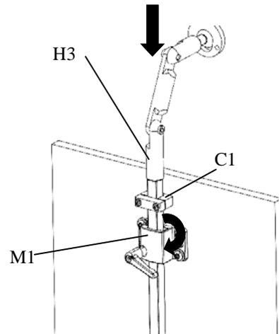
3. Place C1 in desired position and tighten bolts with wrench W2.
