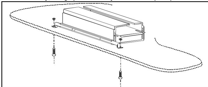
5. Attach the bracket to the tray using appropriate hardware.
