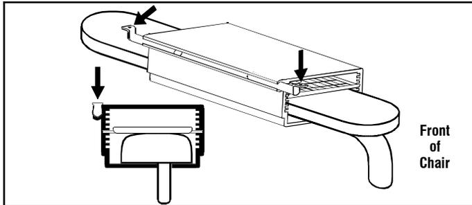
3. Properly position the tray on top of bracket, mark where the holes in **Pivot Pins** make contact with tray. **NOTE: If the tray is padded, you must determine the appropriate way to fasten the bracket to the underside of the tray, and you must supply the fastening hardware of your choice. If the tray is padded, do not follow step 4.**
