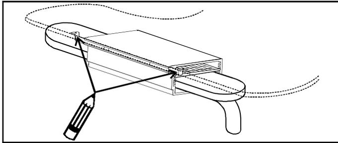
4. Remove tray and flip upside down on a flat working surface. Drill a 1/4" hole through the tray on each pivot pin hole mark. Countersink the holes on top side of tray, so that the socket head screw is flush with the surface of the tray. Remove bracket from armrest and reposition on tray, lining up holes in tray with holes in pivot pins.
