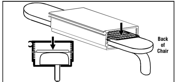
4. The **Snap Tabs** on either side of the **Sliding Spacer** **MUST BE INSTALLED INTO THE SAME SLOT ON EACH SIDE OF THE BRACKET.**
