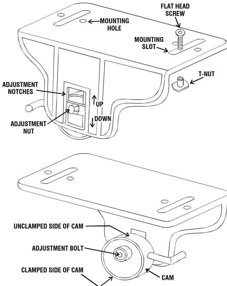
1. Using allen wrench provided, loosen **Adjustment Bolt** so the **Cam** easily slides up and down in **Adjustment Notch** slide. Position clamp onto armrest. With the **UNCLAMPED** side of **Cam** facing the underside of the armpad, push **Cam** up in **Adjustment Notch** slide until the **Cam** loosely contacts underside of armpad.
