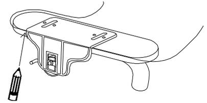
2. Remove tray and flip upside down on a flat working surface. Position clamps on tray, lining up with marks. Using clamps as a template, mark where **Slots** in brackets make contact with tray.
