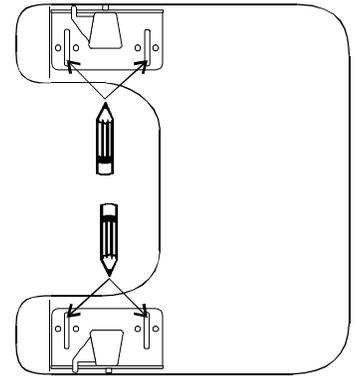
3. Remove clamps from tray, drill one hole through tray in approximate center of each marked slot area. Countersink holes on top side of tray so **Flat Head Screws** will be flush with the tray surface.
